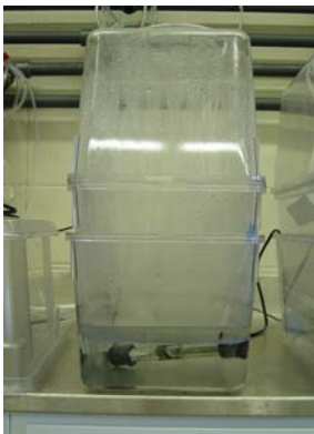
Figure 2.5 Incubator for zebrafish rearing. This is an inexpensive alternative assembled from 3 plastic cages used for rat housing and an aquarium heater adjusted to 28.5°C.
